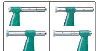
adjust collars for different measuring ranges
