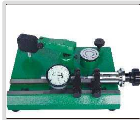
inspect accuracy of dial indicators (range 0-25mm)
