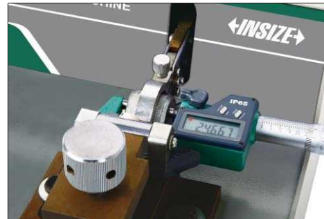
lapping measuring surfaces of outside micrometer
