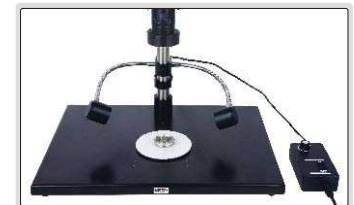
illumination direction and brightness are adjustable
