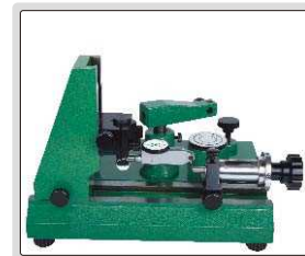
inspect accuracy of test indicators
