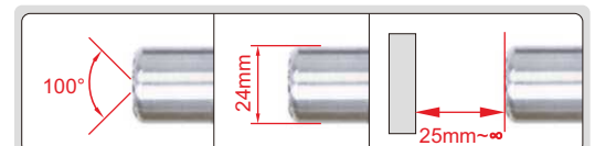
angle of view (θ) diameter (ØD) focus distance (F)
