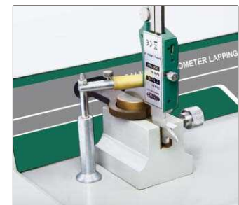
lapping measuring surfaces of caliper lower jaws
