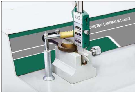
lapping measuring surfaces of caliper lower jaws
