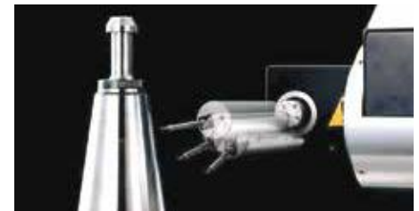
Detector rotation mechanism (0 to 290°, in increments of 1°)
