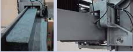
Integrated Y-Axis in Granite Table
