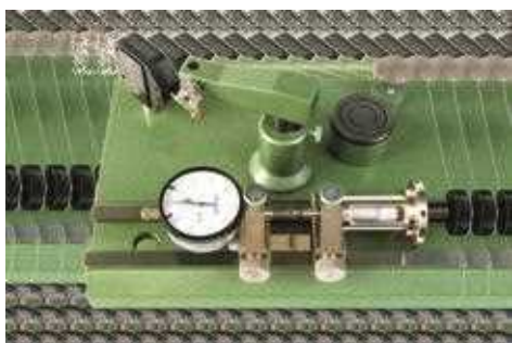
inspect accuracy of dial indicators (range 0-25mm)
