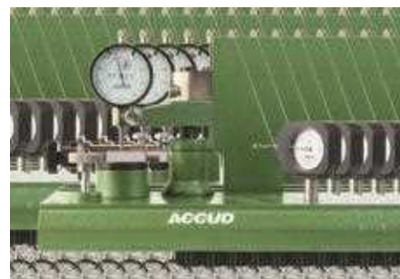
check the effect of lateral force on accuracy of dial indicators
