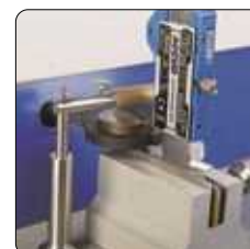
lapping measuring surfaces of caliper lower jaws
