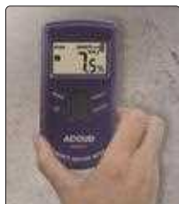
Measure concrete moisture
