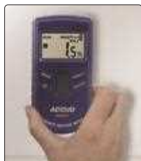
Measure wall moisture
