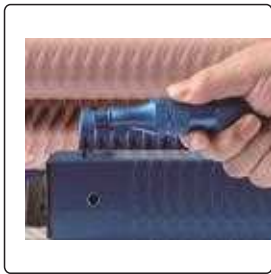
step 1: make grid cutting on surface
